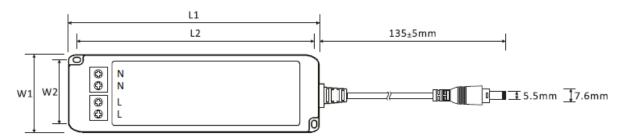
Looping terminals for L and N for easy and quick installation
